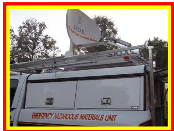
Auto Acquiring 0.95m High-Power Satellite Dish
